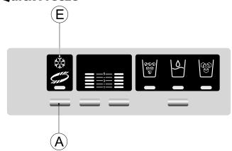
To use the 'Quick Freeze' function, press button A. Indicator E will illuminate to show you that the function is operational. To switch 'Super Freeze' off, press button A again – indicator E will go out.
